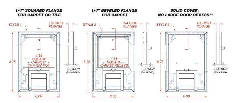
\*\*Note: Cover Shim Kit (FL-200-CSK) may be required to set the height of box "Pre-Pour" so the top of Finish Cover matches top of finished floor.
